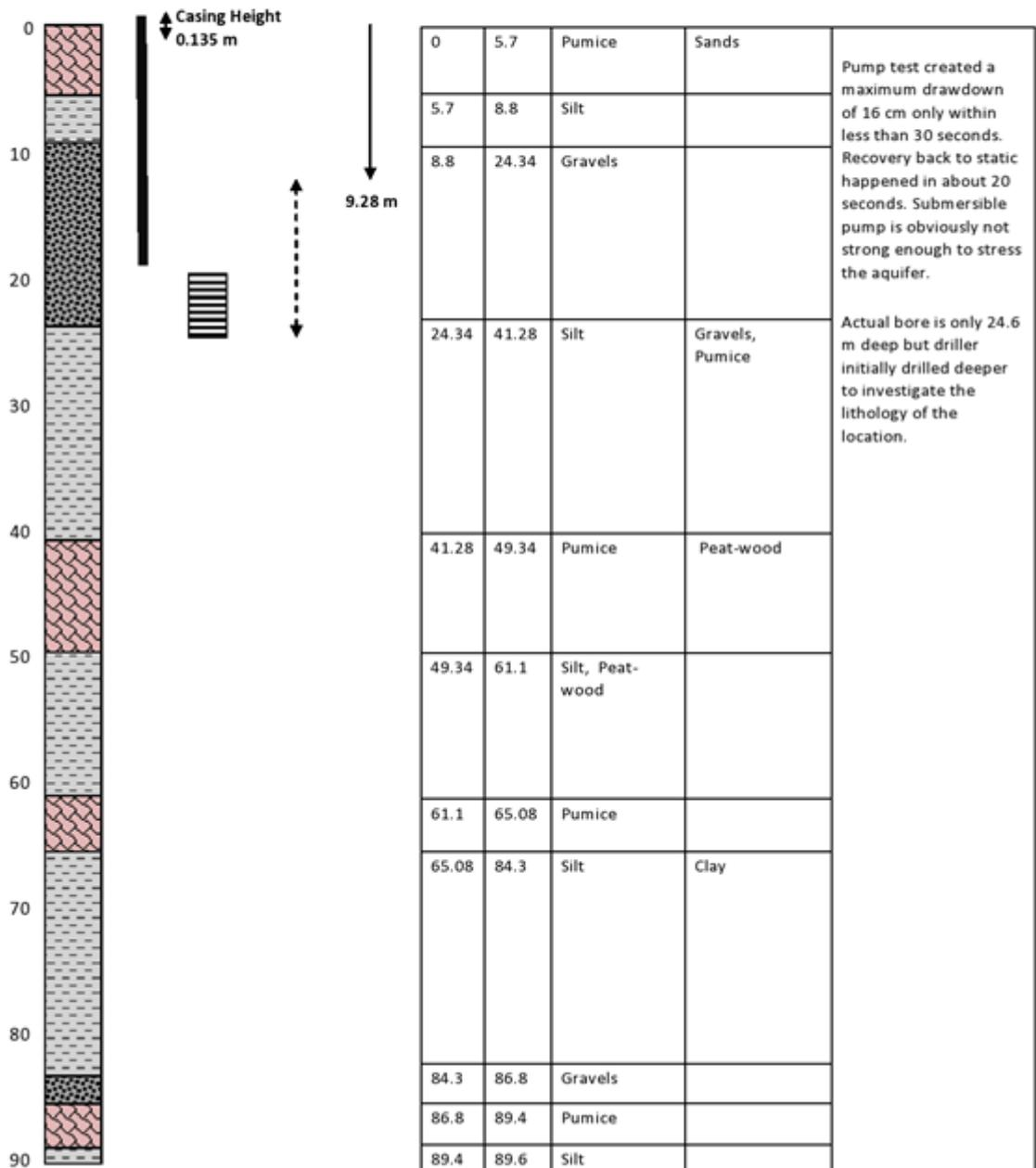
**Pumping test comments for 72\_4014:** A single well test was performed with both drawdown and recovery data collected on the 05/03/2015. The installed pump was not running for at least 12 hours prior to starting the hydraulic test. The pump was forced to run for 90 minutes: the pump rate dropped from 1.23 L/s initially to 1.04 L/s after about 90
