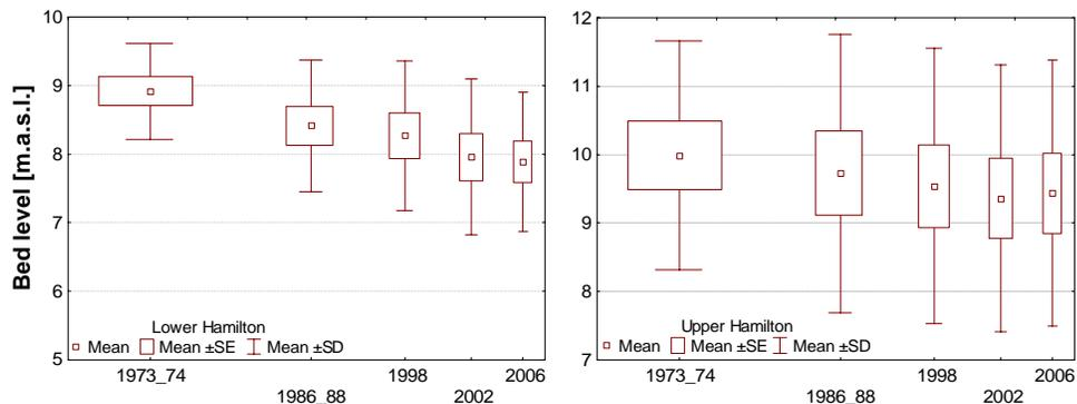
Figure 12 Hamilton City cross section mean bed level statistics from Fairfield Bridge downstream (left) and from Boundary Rd Bridge upstream (right) showing changes with time. SE = standard error, SD = standard deviation of the cross section mean bed level.
