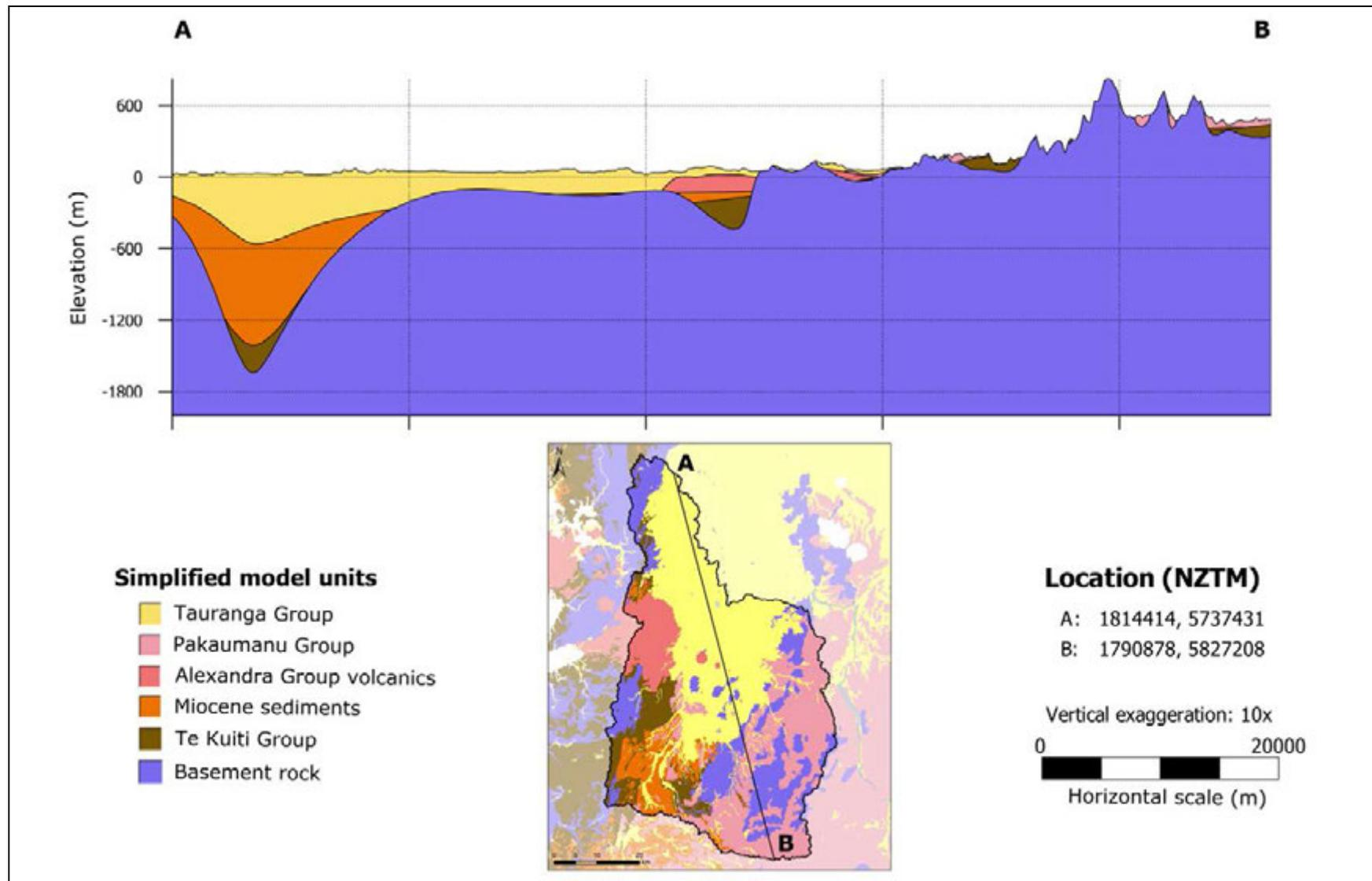
Figure 4.5 North-south cross-section through the Waipa geological model.
