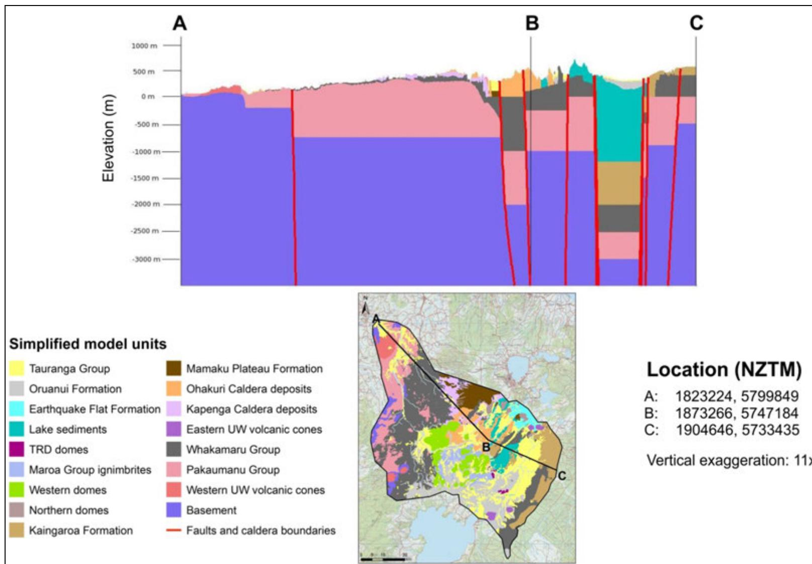
Figure 4.2 North-south cross-section through the UW geological model.
