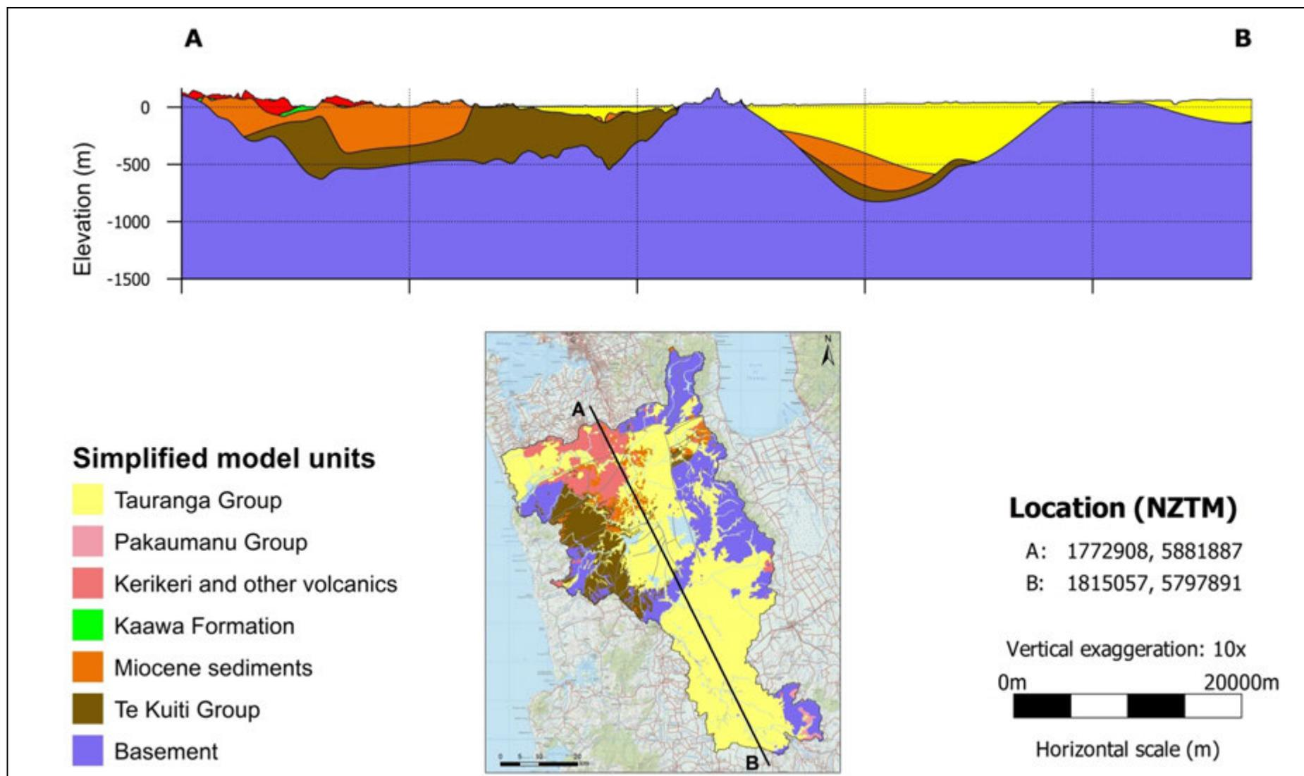
Figure 4.8 North-south cross-section through the LMW geological model.
