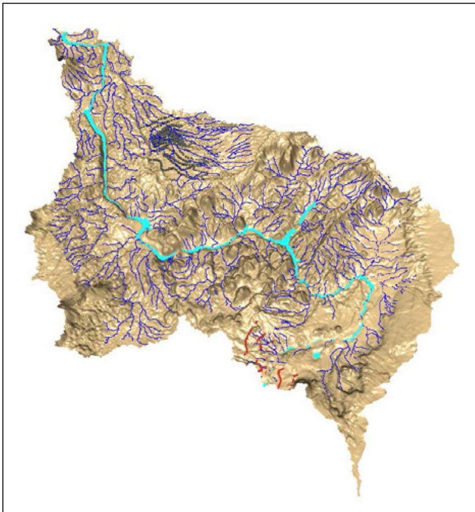
Figure 4.3 Piezometric surface of the UW zone at 10x elevation exaggeration. The following datasets have been added for comparison purposes: piezometric contours in purple (Waikato Regional Council, 1991); piezometric contours in grey (Waikato Valley Authority, 1987); piezometric contours in red (Bromley *et al.*, 2000); fixed-head cells in light blue for Lake Rotokawa and the Waikato River; and fixed-head cells representing streams in dark blue. The view direction is towards the north.
