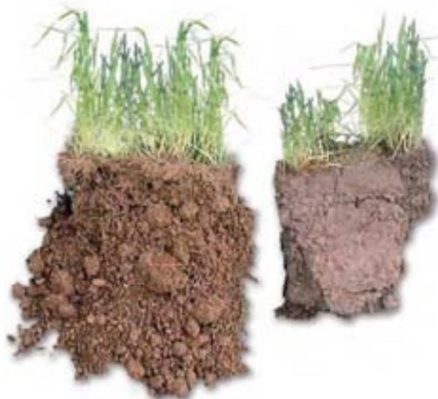
An uncompacted topsoil on the left contrasts with the compacted soil on the right.
