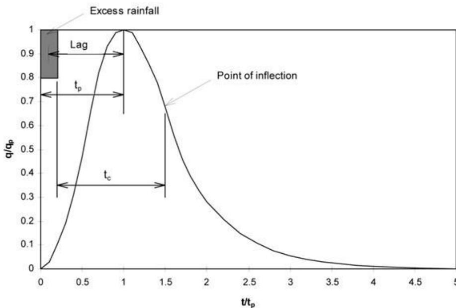
Figure 6-1:Figure 2-2: NRCS unit hydrograph (previously shown as Figure 2-2)<sup>23</sup>
