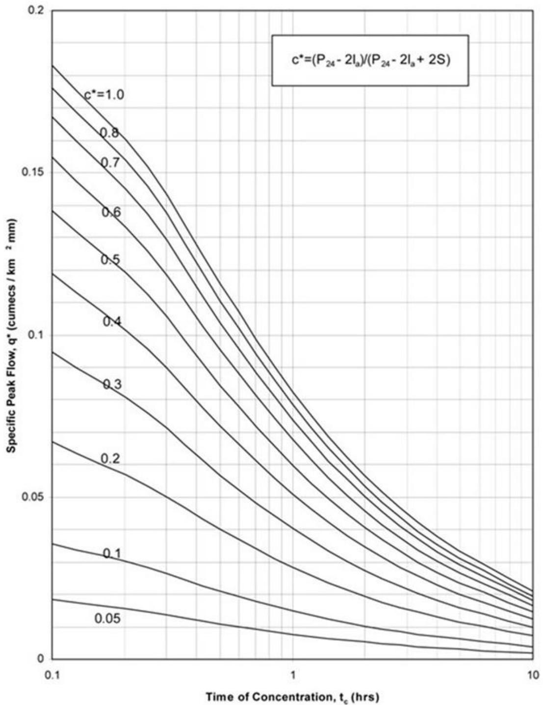
Figure 8-1: Determining the specific flow rate<sup>32</sup>
