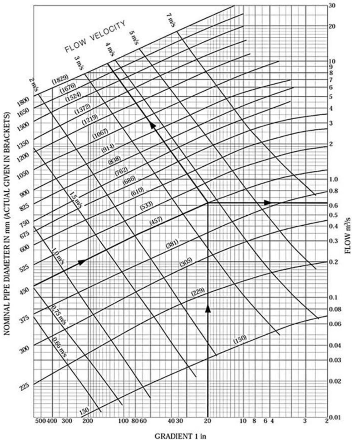
Example: a 450 mm internal diameter pipe with a gradient of 1 in 20 will have a flow of 0.63  $m^3/s$  at a velocity of 3.75 m/s
