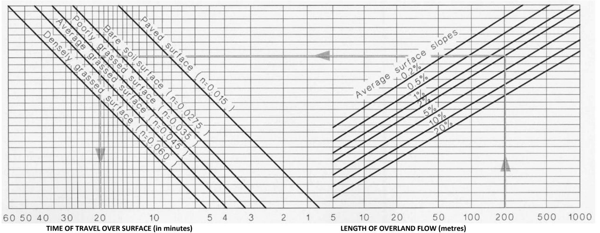
Example: For surface water flowing 200 m over an average grassed surface at a slope of 2% the time of travel is 20 minutes
