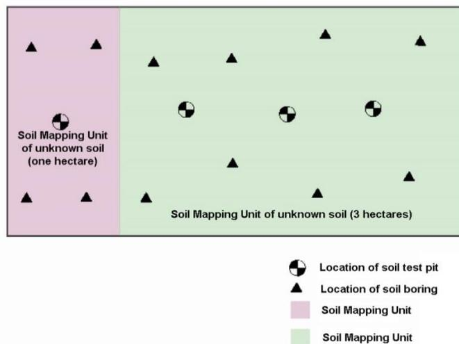
**Figure 5-1: Indicative soil testing site arrangement**
