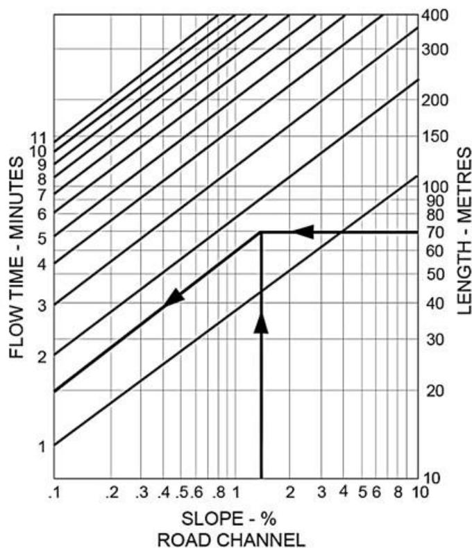
**Example:** For a slope of 1.4% and a road channel length of 70 metres the time of road channel flow is 1.7 minutes
