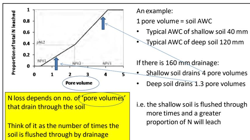
**Figure 1.** Shape of N leaching curve as derived by Cichota et al (2012). NPV ('number of pore volumes') values denote start of leaching (nPV1) an inflexion in the linear relationship between pore volumes drained and proportion of N leached (nPV2) and number of pore volumes required to complete leaching (nPV3). These values vary with soil type
