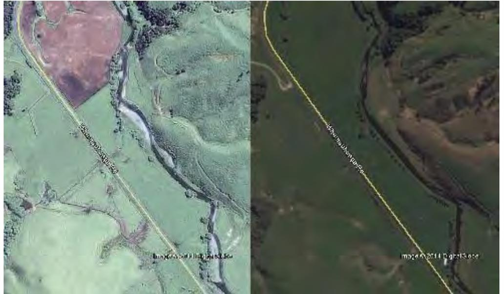
Figure 9. Left 2000 and right 2013 showing the removal of gravel bars and straightening of the Mangatutu River.
