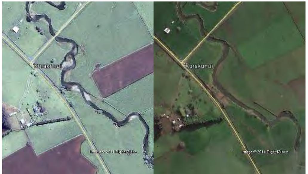
Figure 8. Left 2000 and right 2013 showing the removal of gravel bars and straightening of the Mangatutu River.
